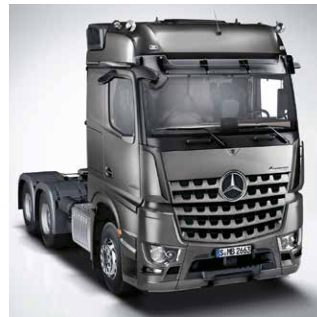
BigSpace L-cab . With standing headroom of 1.99 m between the seats, the cab with a level floor and measuring 2500 mm in width offers unusually generous freedom of movement and comfortable through-access to the co-driver's side.
