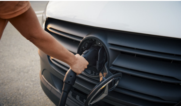
CCS rapid charging port, 115kW max. capacity.
