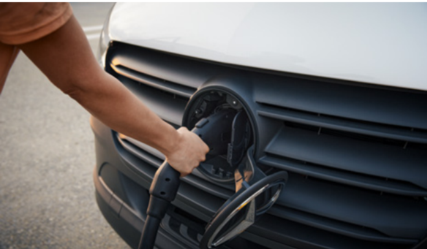
CCS rapid charging port, 115kW max. capacity.
