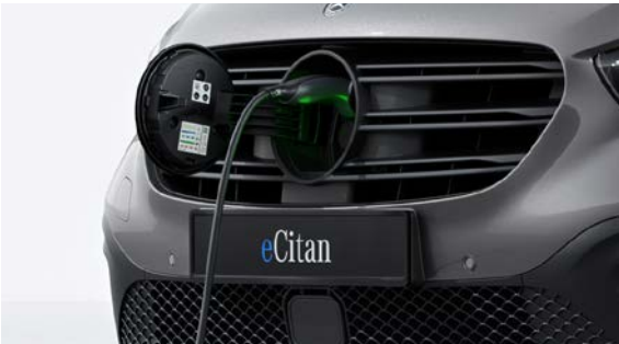
CCS rapid charging port, 75kW max. capacity.
