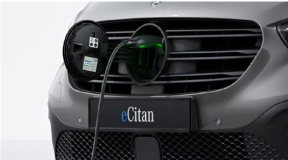
CCS rapid charging port, 75kW max. capacity.
