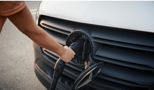
CCS rapid charging port, 115kW max. capacity.
