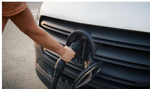
CCS rapid charging port, 115kW max. capacity.
