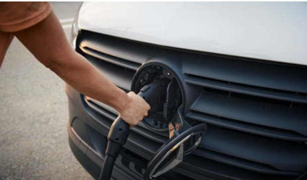
CCS rapid charging port, 115kW max. capacity.
