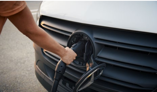
CCS rapid charging port, 115kW max. capacity.
