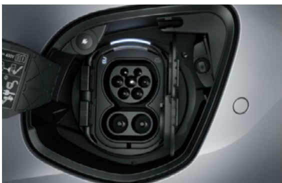
CCS rapid charging port, 80kW max. capacity.
